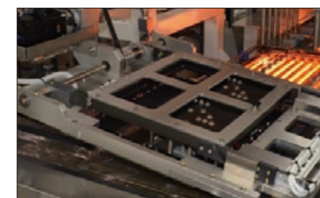
可设定各种浸焊条件 Various dip soldering can be set
