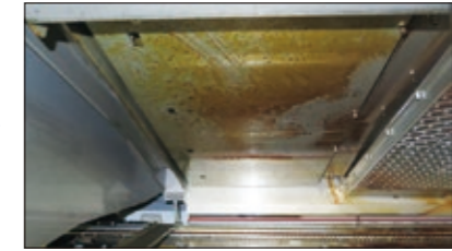
助焊剂回收系统OFF状态 Flux management system OFF
