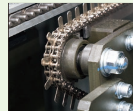
防基板翘曲机构 PCB warpage prevention mechanism
